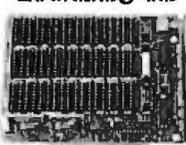
**Expansion Memory Half-Card for IBM-PC, XT, Portable, Tandy 1200 and Compatible Computers**
