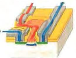
How a transistor operates as a switch.
