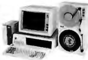
Now you can exchange data files between your IBM PC/XT/AT and any mainframe or minicomputer using IBM compatible 1600 BPI 9-Track tape. Unit can also be used for disk backup and archival storage. Transfer rate is one megabyte per minute on PCs and 100% compatibles. Subsystems include 7" or 10 1/2" streaming tape drive, tape coupler card and DOS compatible software.
