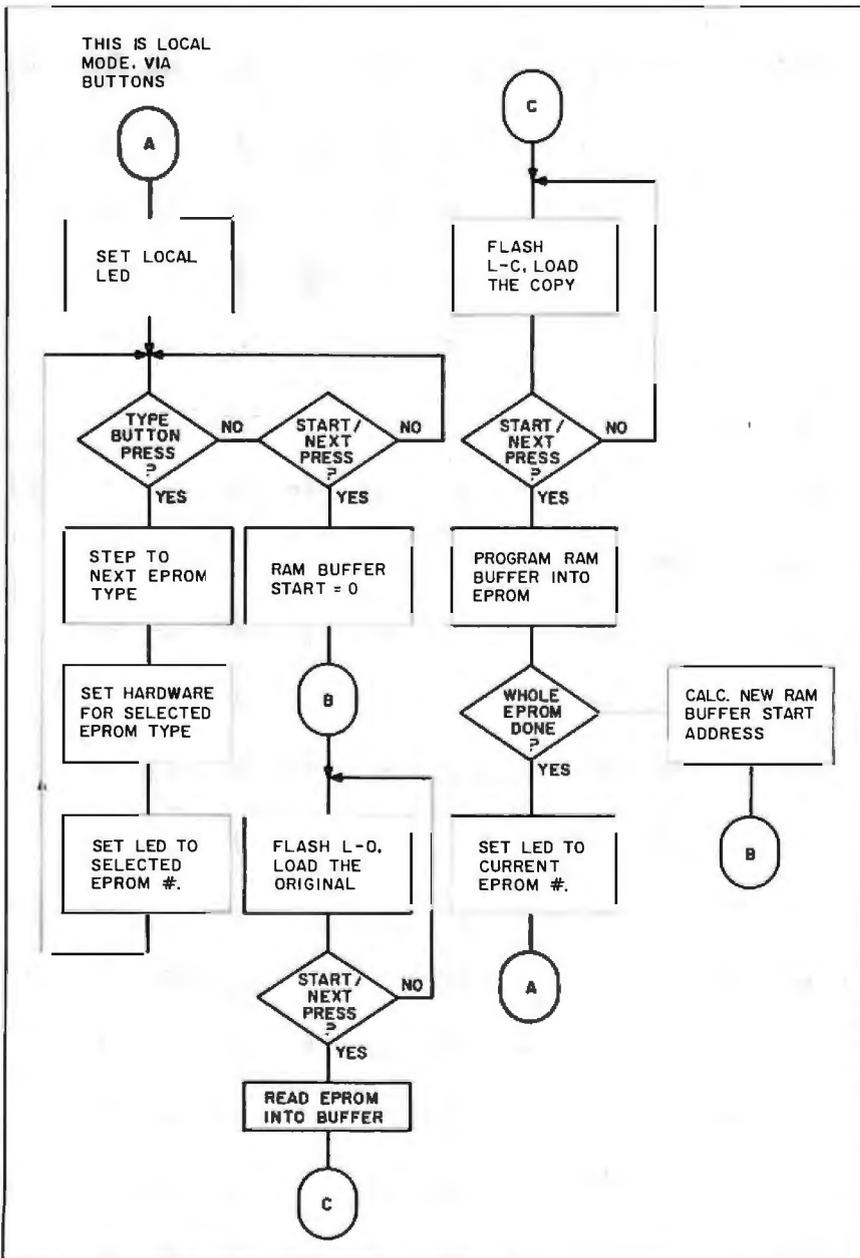
Figure 7c: Flowchart 3, logic flow for the local mode.
