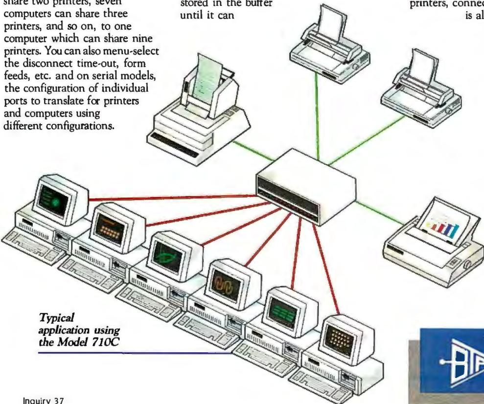
Typical application using the Model 710C
