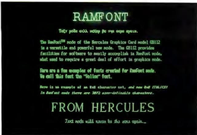
The Graphics Card Plus in RamFont mode showing multiple fonts created using FontMan,™ a Hercules program that comes free with each Card.
