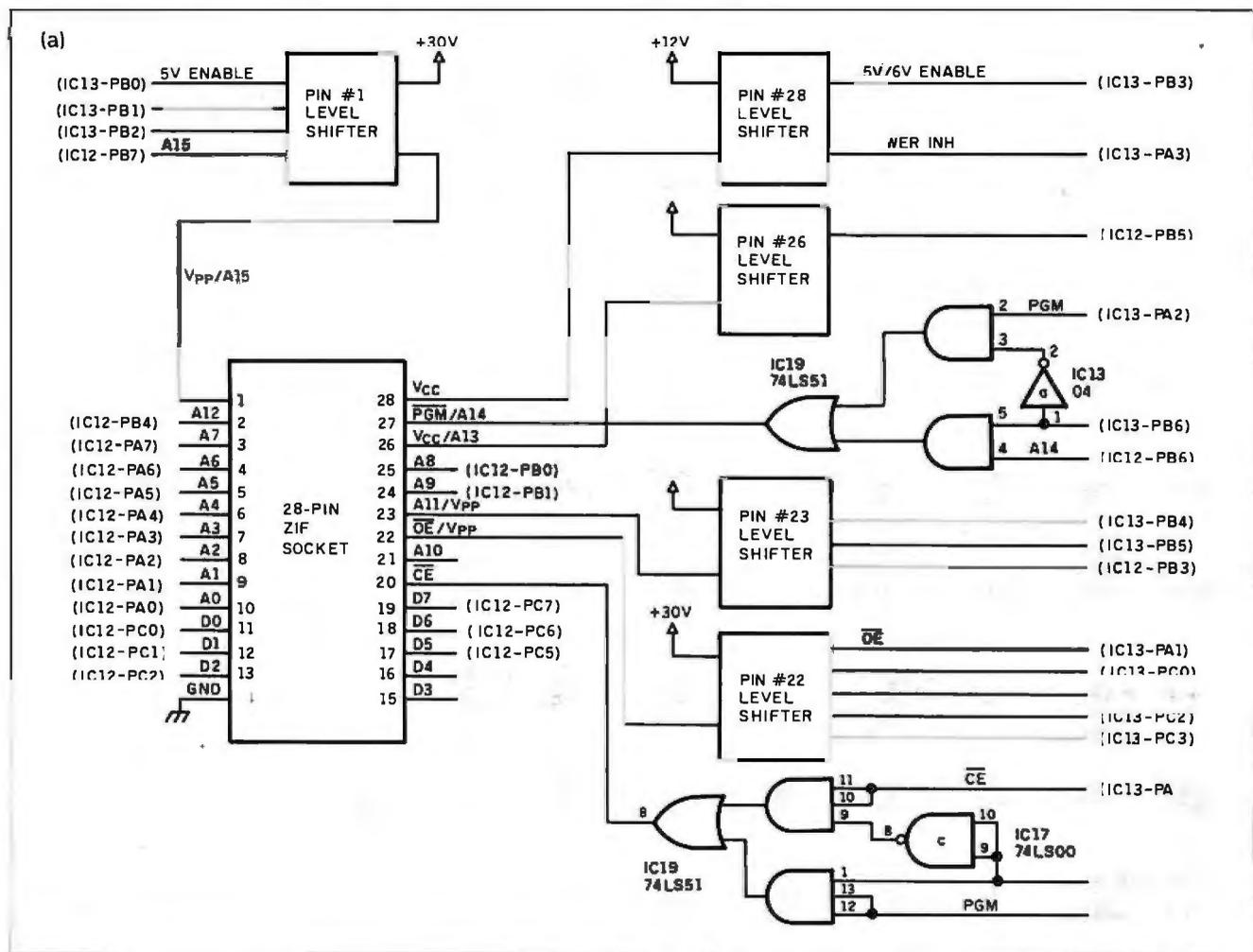
Figure 3: (a) Block diagram showing the connections to the ZIF socket. Note the level-shifter circuitry connections for those pins that require programming voltages or that differ across EPROM types.
