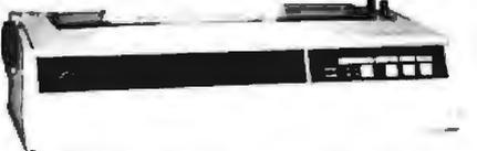
The Adeus CP/2000, is a 22 character per second daisy wheel printer which accepts 96 character Diablo wheels and ribbons. This printer was manufactured by the Olympia Typewriter Company for Cosmo World USA. This unit will print 10, 12 and 15 characters per inch proportionally spaced with increments of 1/120". Bi-directional printing, 2 KByte buffer (expandable to 6K) and both serial and Centronics parallel interfacing make the Adeus CP/2000 an exceptional buy at only \$159. Original price \$595.
